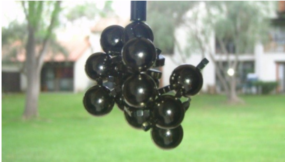
Self Assembled Sculpture in Zero Gravity Third Test. Using Neutral Spheres and Small Cubic Magnets.
